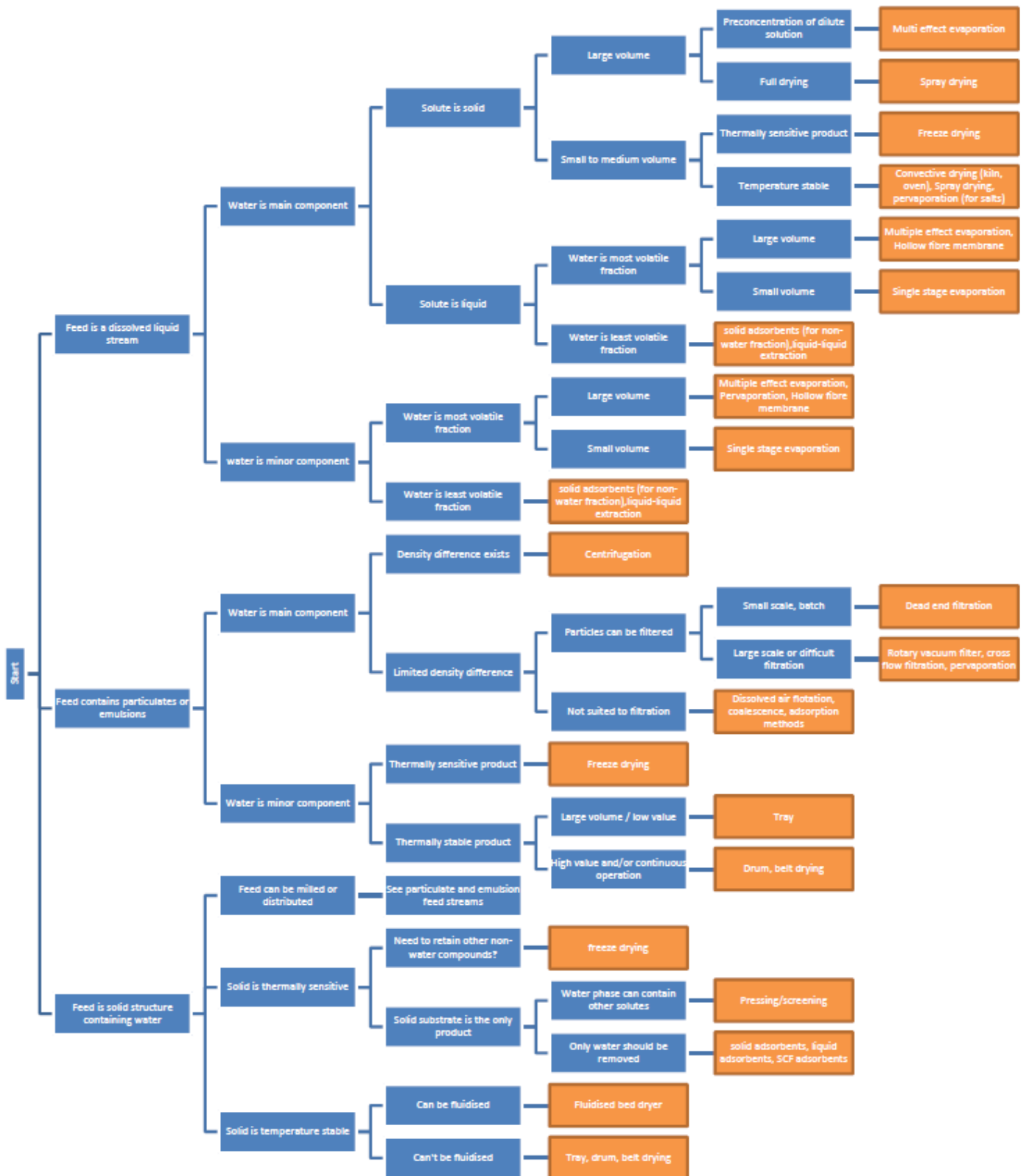
Figure 7.2 – Process selection map. Some process options identified may only be applicable for specific sub-applications, or be dependent on availability of a suitable solvent or adsorbent. Processing steps may also be used in combination – for example water content reduction by falling film evaporation followed by a final drying step suited to a viscous or solid final product.
